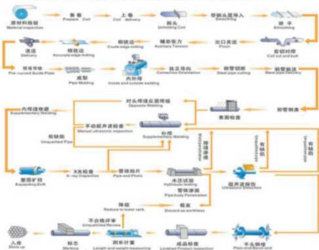
螺旋焊管生产工艺流程图 SSAB steel pipe production process flow chart
